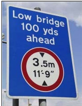
Photo: Sign layout at key junctions on the approach to a low bridge with regulatory signs
