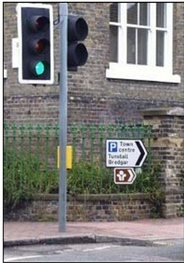
Photo: Signs mounted on railings (with owner's consent) to reduce clutter and visual intrusion
